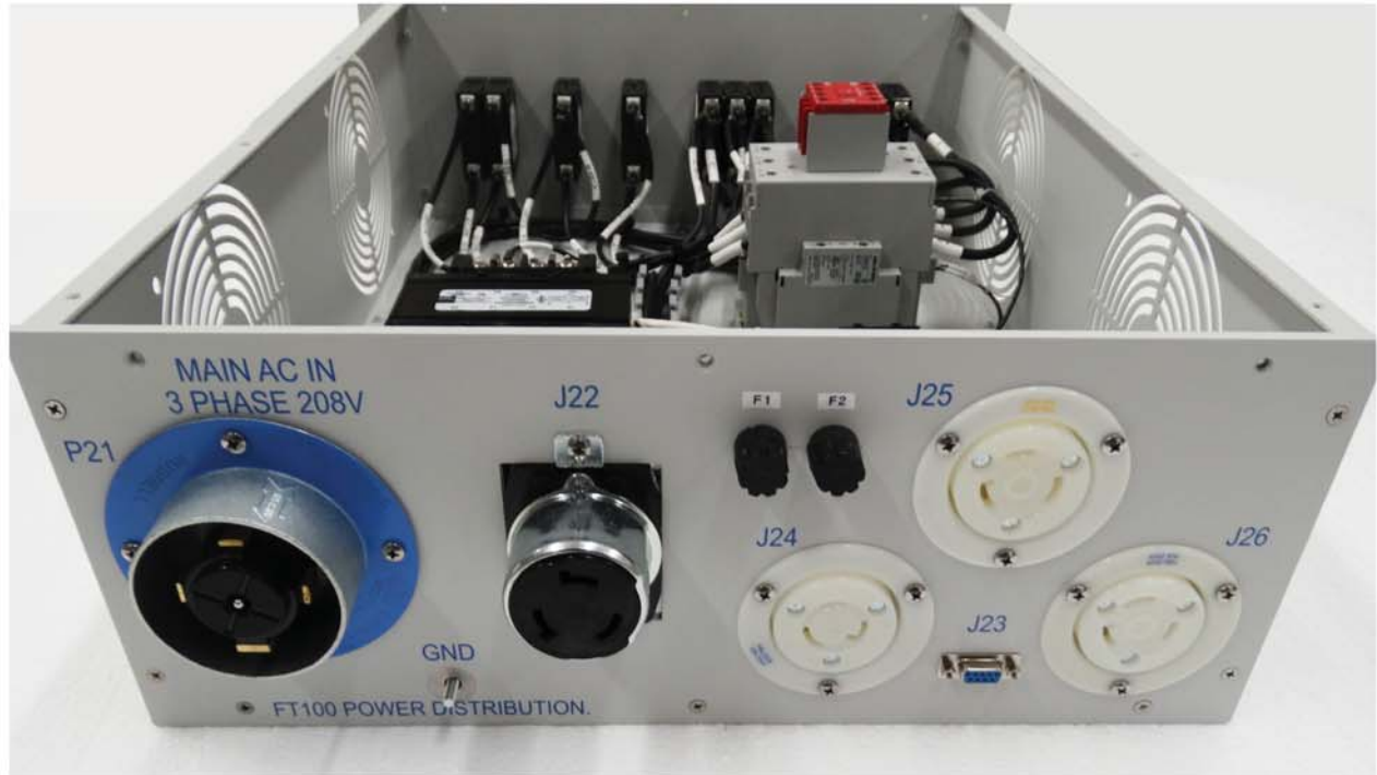
Rear View with cover removed showing Input and Output AC Connectors
