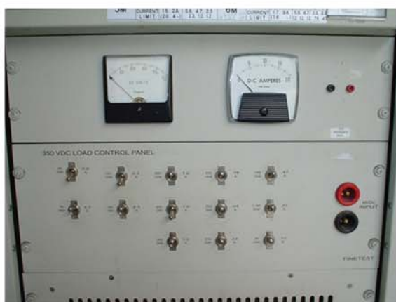
Close-Up of Load Value Switches DC Voltage and Current meters and Load Input Connectors
