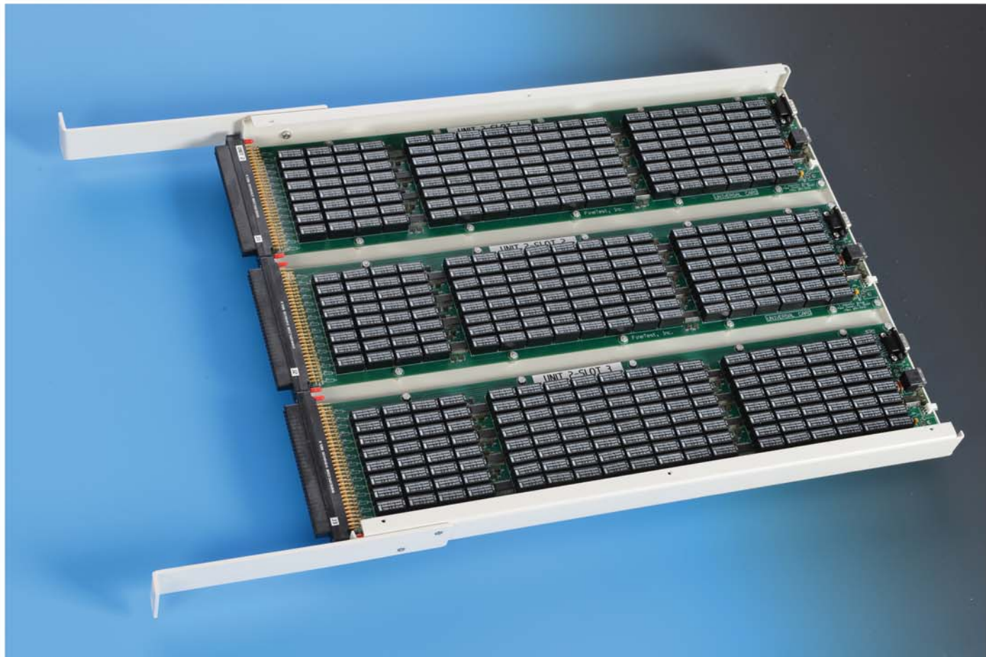
Cover removed showing 3 16x9 Cards
