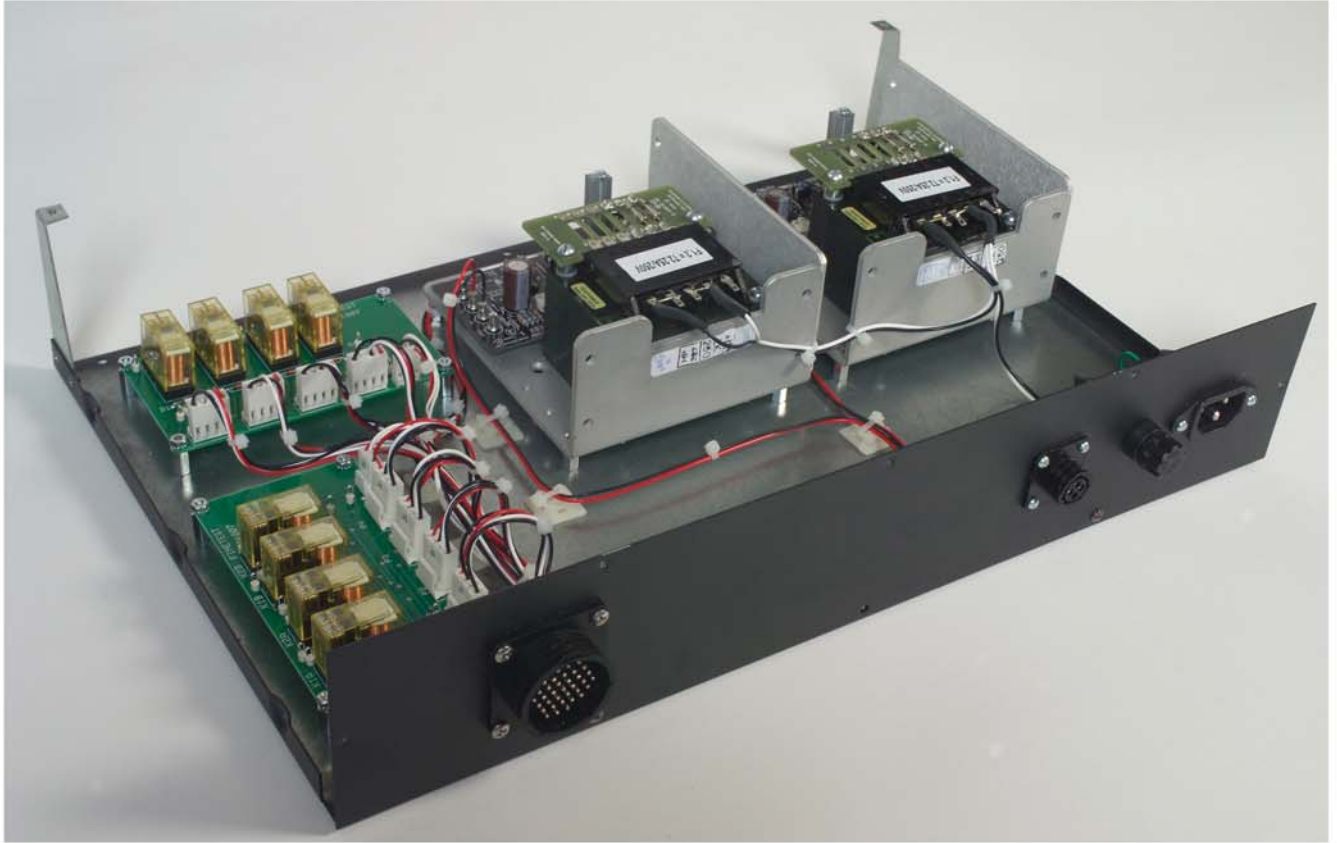
Rear Angle view of DC Mux Unit with front and cover removed
