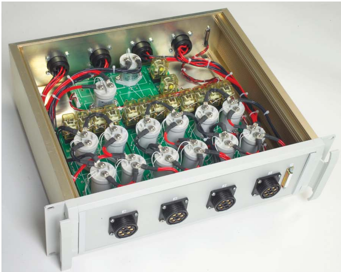
Top View with Cover Removed showing High Voltage/ High Current Power Relays
